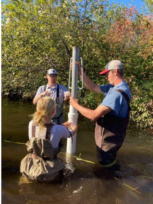
Left: North Ed Career Tech students Bailey Ray, Mancelona High School senior, and Thomas Mckee, Kalkaska High School junior, pound a PVC pipe into the riverbed and use a tape measure equipped with an electronic probe that emits a loud beep when it comes in contact with water.
