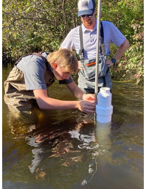
Left: North Ed Career Tech students Bailey Ray, Mancelona High School senior, and Thomas Mckee, Kalkaska High School junior, pound a PVC pipe into the riverbed and use a tape measure equipped with an electronic probe that emits a loud beep when it comes in contact with water.
